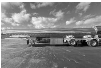
'24 Wabash non-code DEF trlr. , S.S. insulated, air ride, spread axle, 5000-gal. cap.
