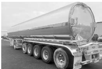
'25 Tremcar DOT 406 , alum. barrel, S.S. frame, 13,400-gal., 5-compt., air ride, disc brakes, leasing available.
